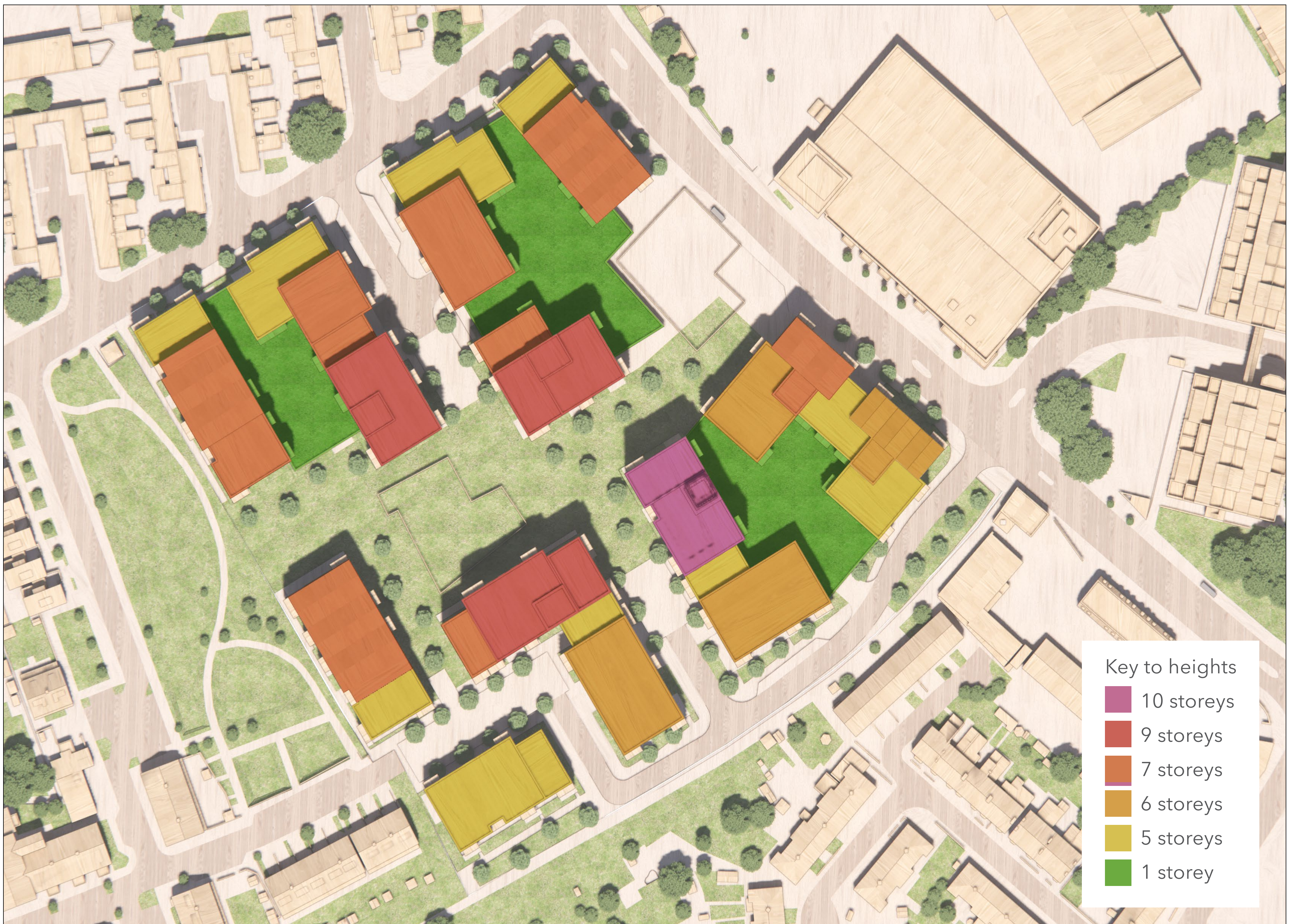
Roof plan showing the height of the proposed new buildings in storeys
